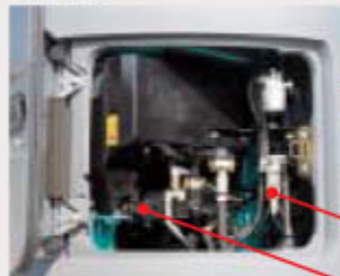
Large fuel filter (with built-in water separator)/Water separator
