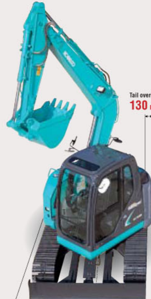
Min. front swing radius: 1,760 mm Tail swing radius: 1,290 mm
